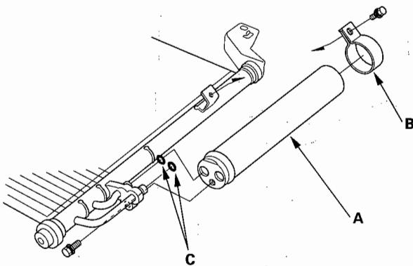
3. Install the receiver/dryer in the reverse order of removal, and note these items:
